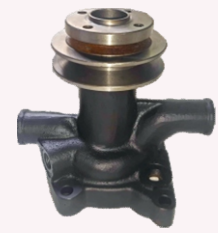
INDOFARM TRACTOR LOADER (PULLEY DIA 97MM, FAN COLLAR 34MM)
